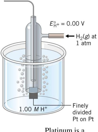
The standard hydrogen electrode. Hydrogen gas at 1 atm is passed over finely divided platinum. The solution contains 1.00 *M* hydrogen ion. The reduction potential is exactly 0 V at 298 K  $(25^{\circ}C).$
