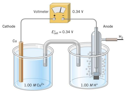
A galvanic cell comprised of copper and hydrogen half-cells. The reaction is  $Cu^{2+}(aq)+H_2(g) \rightarrow$  $Cu(s)+2H^+(aq)$
