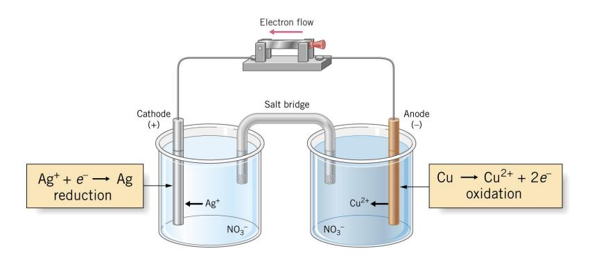
A galvanic cell. The cell consists of two half-cells where the oxidation and reduction half-reactions take place. The salt bridge is required for electrical neutrality. The overall *cell reaction* is:  $2Ag^+(aq)+Cu(s) \rightarrow 2Ag(s)+Cu^2+(aq)$
